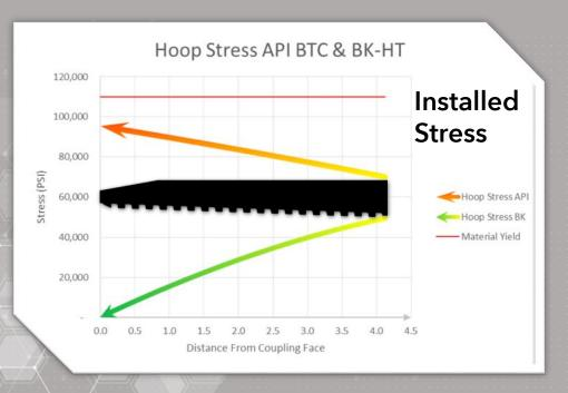
The coupling will return to its original shape after the frac without high residual stresses and deformations that accelerate corrosion and crack growth.
