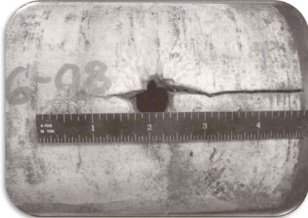
The pin tooth crest can ride on top of the box tooth crest past the coupling center; the cross threading leads to a crack initiated washout.
