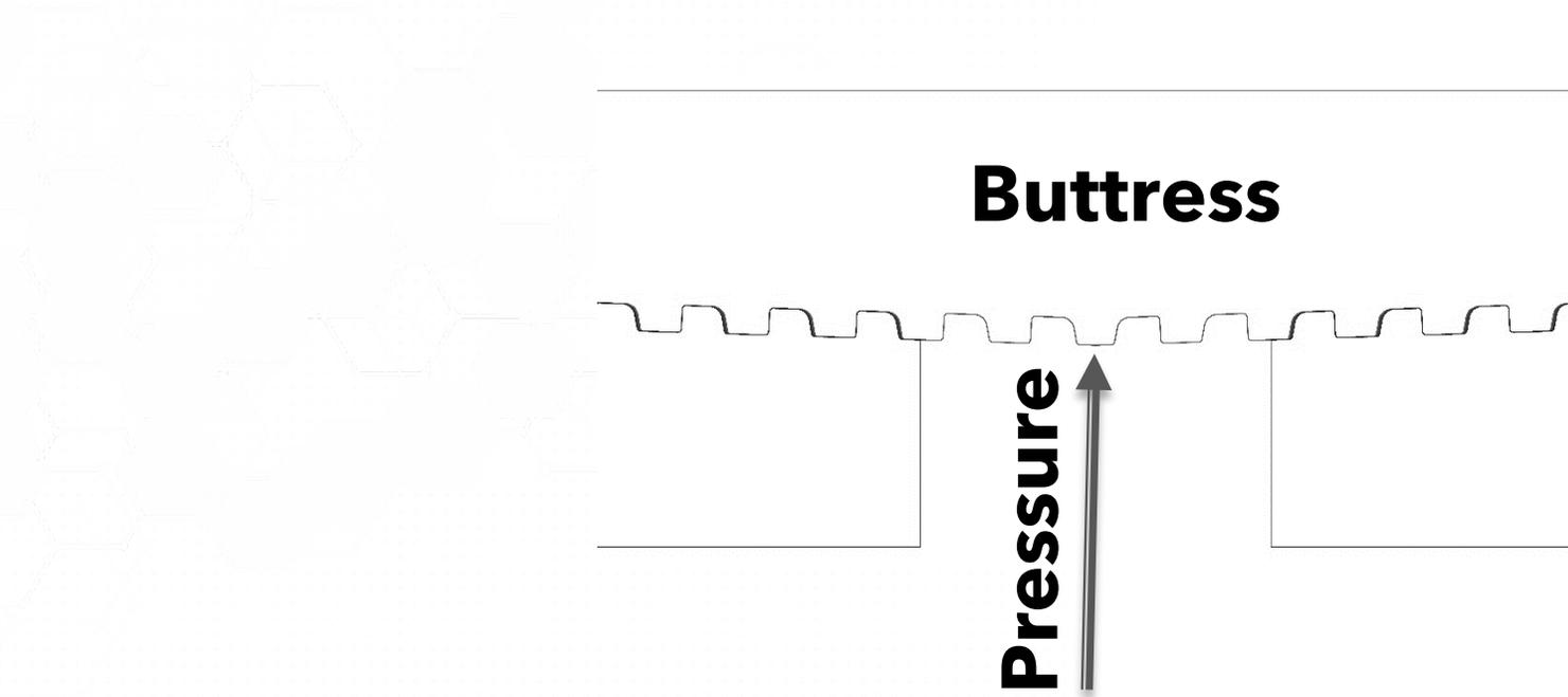
Standard Buttress allows the internal pressure to react against the thin walled coupling.
