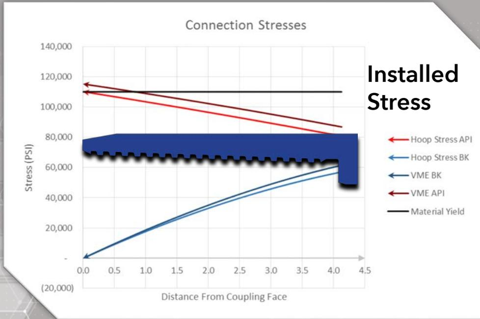
*The coupling will return to its original shape after the frac without high residual stresses and deformations that accelerate corrosion and crack growth.*
