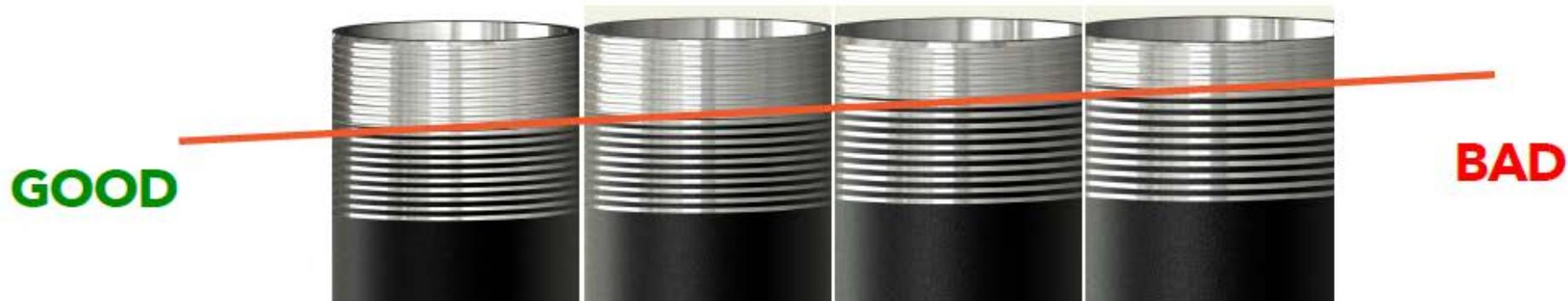
**\* Black Crested Threads provide a leak path.**
