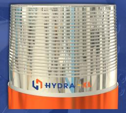
The HYDRA-XL utilizes a patented advanced square stepped thread design for a deep easy stab. The box and pin threads are asymmetric run-in / run-out threads that maximize the critical section area available for pull strength. Square threads are used because of their flexibility in a bend and ability to absorb high tensile and compressive loads.
