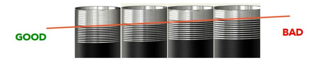
Black Crested Threads provide a leak path.
