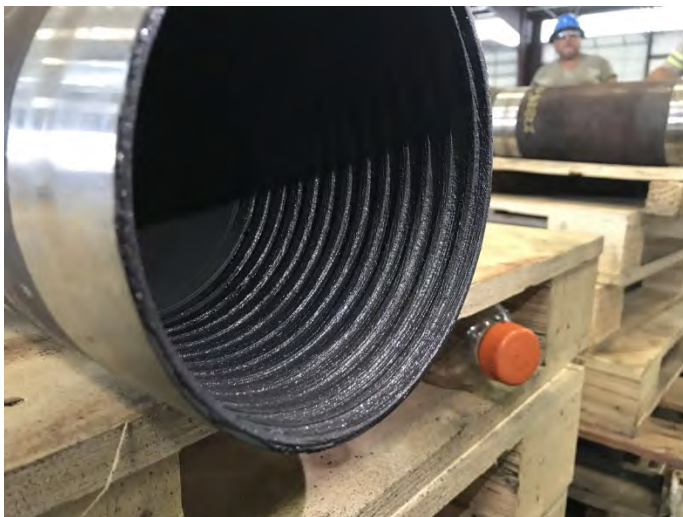
Thread compound on box only with tradition thread compounds such as BOL 2000 or similiar
